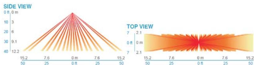
The image above shows the coverage pattern for the Sensor Switch Aisleway occupancy sensor. This sensor has a special lens that directs coverage on the aisleway instead of areas with racking. The segments of the lens also enhance the coverage of the sensor so that fewer units can be used in an aisleway application
