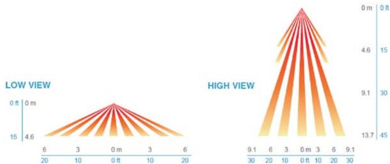
The image above illustrates the coverage pattern for a high bay occupancy sensor with a 360 degree field of view. This device looks down from either the high bay fixture or the junction box that it is mounted on, and covers a circular area extending out from the point directly below the mounting position. The size of this circle depends on the mounting height.
